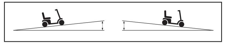
Figure 2. Maximum Allowable Incline Angle (Ascending and Descending)
